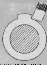
SQUARENOSE TOOL FOR FINISH CUT
